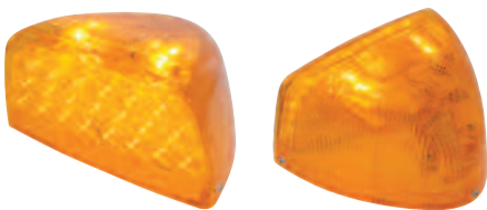
Only Front and Top LEDs Lit on Dim During Running
